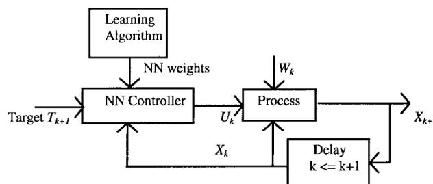
Fig. 1. Block diagram of the DA SPSA neural network-based control system.
