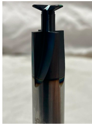
Figure 1. The custom four-flute form keyseat cutter used to modify the mirror hanger on DART's DRACO instrument. To prevent damage to DRACO's mirror during launch, APL's fabrication team collaborated with the engineering team to design a custom tool that was used to modify the mirror's hanger to maximize its flexibility.
