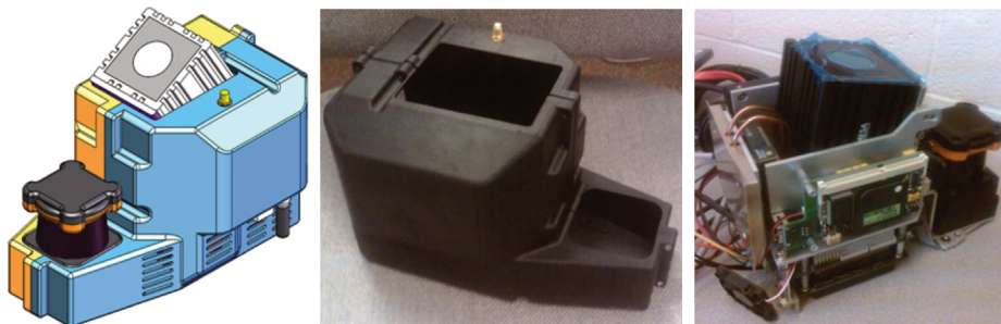
Figure 3. EMAPS backpack-mounted mapping sensor head version 1. Initial prototypes incorporated quick-turn sheet metal components and heatsinking plates to support and dissipate heat from the COTS electronics and imaging systems.
