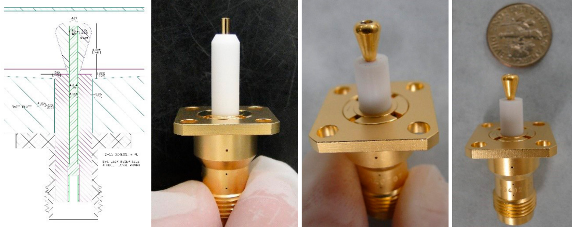
Figure 14. RLSA for the DART mission. The radiator cone can heat up to over 200°C during operation, requiring a high-temperature solder to reflow attach the cone. In addition, the insulation and center pin lengths of the original connector were modified. The small cone was machined in APL's machine shop and gold-plated in the microelectronics fabrication lab. Special mechanical fixtures were also made to facilitate the modification and solder reflow attachment of the cone to the center pin.
