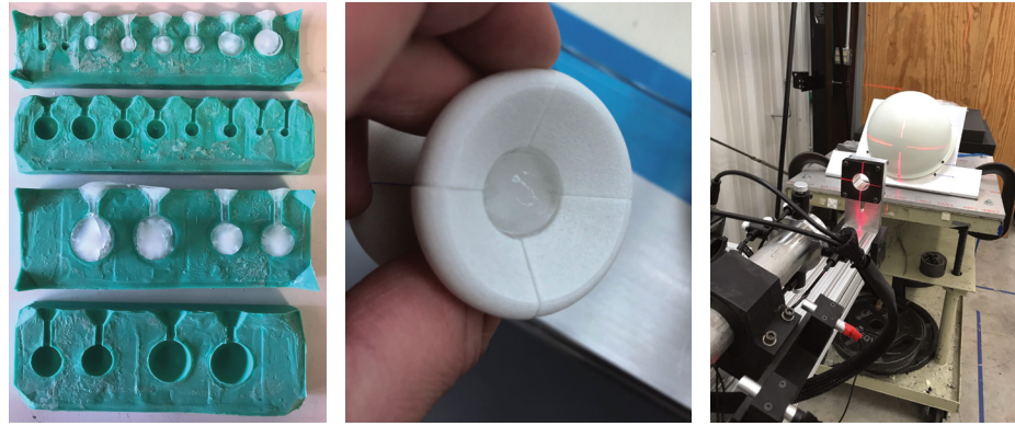
Figure 7. Hail strike simulation to test radome resilience to damage. The team tested simulated hail strikes at various speeds using a silicone mold filled with ice to simulate hailstones (left). The ice was loaded into additively manufactured sabots (center), and an air cannon delivered the simulated hailstones to the radome (right).
