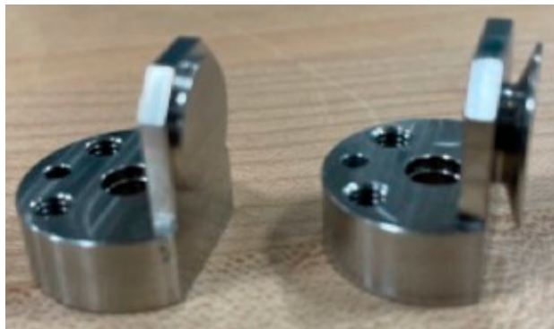
Figure 3. Before (left) and after (right) of the DRACO mirror hanger. The rapid deployment of the redesigned part allowed the spacecraft to pass vibration testing and maintain its scheduled launch date.
