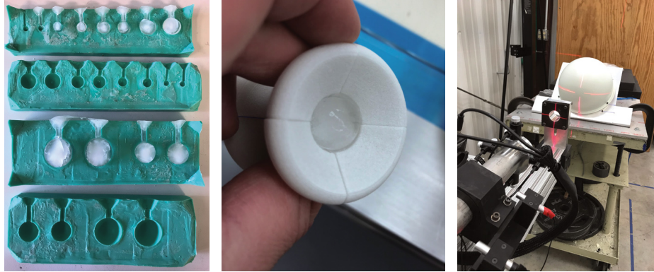
Figure 7. Hail strike simulation to test radome resilience to damage. The team tested simulated hail strikes at various speeds using a silicone mold filled with ice to simulate hailstones (left). The ice was loaded into additively manufactured sabots (center), and an air cannon delivered the simulated hailstones to the radome (right).
