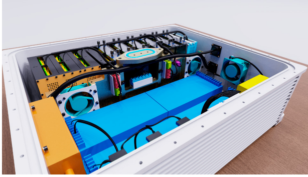
Figure 1. MCAD assembly featuring complex cabling harness. This design was created using the APL-developed WRLpool GUI and helped the MCAD designer account for over 400 conductors in the electronics enclosure.
