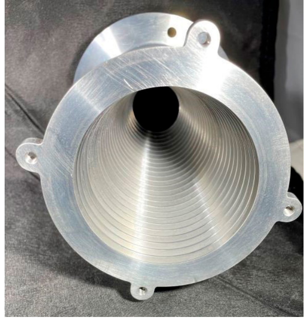
Figure 9. IMAP medium-gain antenna feed horn. To create the grooves on the inside walls, this part was fabricated using a custom groove tool on an advanced multiaxis turning machine.
