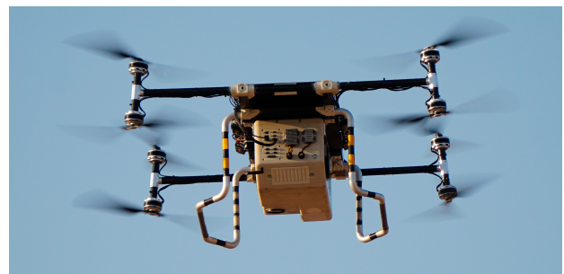
Figure 3. Dragonfly test UAV during flight test. The test vehicle is an approximately half-scale version of the Dragonfly lander, designed and fabricated at APL. It weighs 43.2 kg and measures 1.3 m × 1.2 m × 1.2 m, including the rotor arms, landing skids, sensors, batteries, and computing elements.
