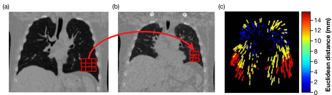
Figure 2. Intuition behind registration. The voxels in the inhalation scan (a) are spatially aligned with those in the exhalation scan (b; red arrow). The output is a deformation field representing the per-voxel vectors that approximate the transformation from the inhalation to exhalation scan. (c) The inverse deformation field (from exhalation to inhalation).
