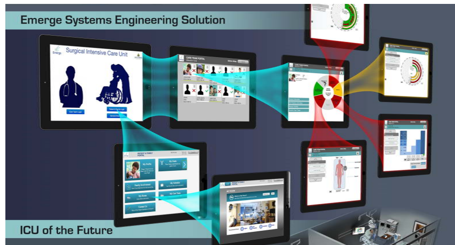
Figure 4. Project Emerge system concept. The system centers on a tablet application that displays integrated data from the various information systems and patient monitoring equipment used in an intensive care unit (ICU). The application's "harms monitor" seeks to reduce the occurrence of seven common preventable harms facing ICU patients by tracking whether preventative measures have been taken.
