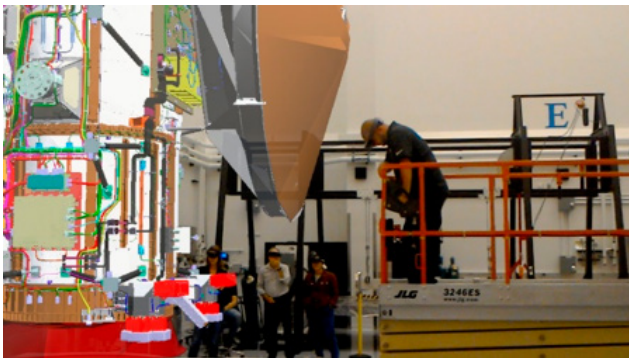
Figure 9. Left, A technician drives the scissor lift to align with the edge of the AR model, creating the distance available for I&T operations. Right, A technician elevates the scissor lift to clear the propulsion module solar array struts and performs a “reach analysis” to assess accessibility to the RF waveguide and connector interfaces.
