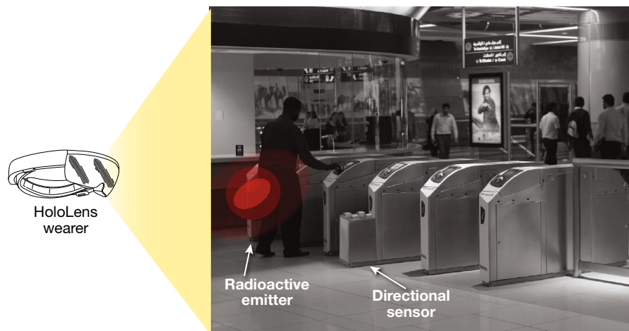
Figure 8. Directional radiation sensing is achieved by binding together multiple sensors and noting the differences among their readings. An agent equipped with the Novel Perception system, which is small enough to be carried in a backpack, mounted on an unmanned vehicle, or placed in a turnstile, would be able to visually scan the environment for hot spots indicating radioactivity and quickly assess the location, extent, and concentration of emissions in real time as an augmented reality overlay.
