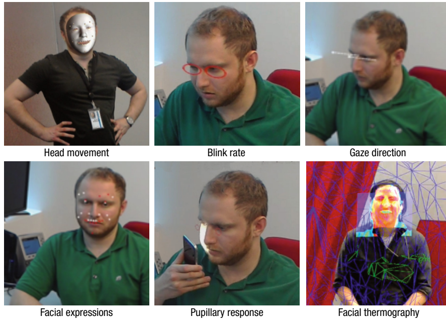
Figure 6. Social vision. This modality enables finer perception of nonverbal cues. The user wearing the headset is able to view data points overlaid on the interaction partner’s face, enabling the headset wearer to receive information in a way that is easily interpretable, in real time, and without interrupting the social interaction.
