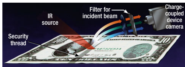
Figure 8. Noncontact probing of currency by using a laser or light beam focused on a phosphor-infused security thread in a paper note. (Reprinted from Ref. 17.)
