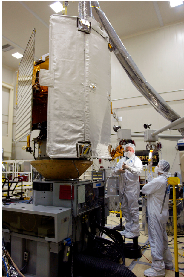
Figure 5. MESSENGER engineers at APL adjust the ceramic-fabric sunshade in preparation for the spacecraft vibration test.
