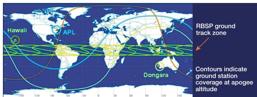
Figure 4. Ground station location and fields of view at apogee distance. Note that at closer distances, the coverage area diminishes; however, the closer distance enables a higher downlink rate for increased data volume throughput.
