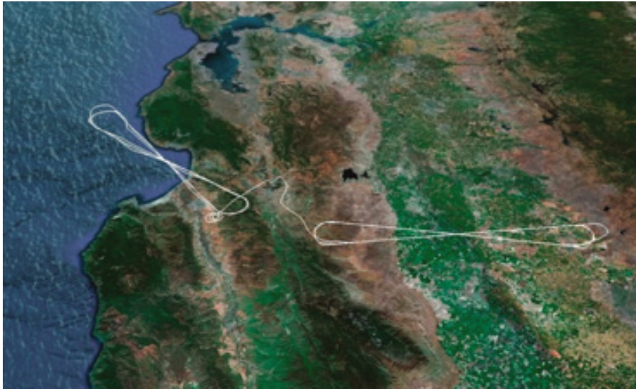
Figure 15. Flight pattern used for air-to-air testing. The maximum range between the aircraft was 230 km.
