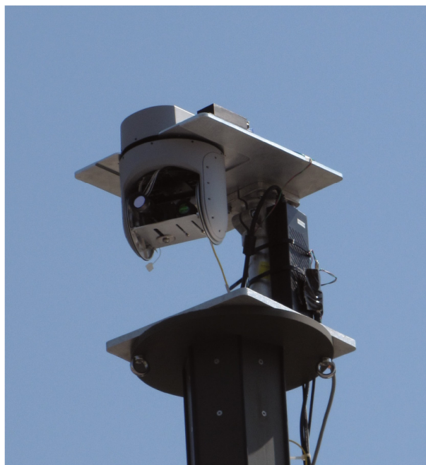
Figure 24. Prototype compact lasercom terminal on a deployable mast during outdoor tests.
