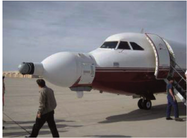
Figure 3. DARPA ORCA test aircraft. The lasercom terminal is at the tip of the aircraft nose.
