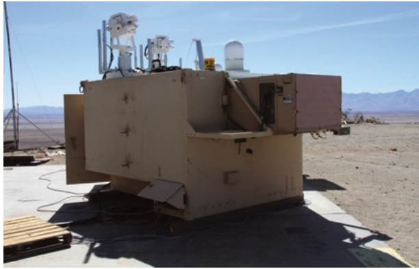
Figure 10. Test configuration of the FOENEX ground station at China Lake Naval Air Weapons Station. Shown are the two lasercom and RF terminals.
