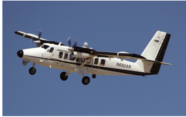
Figure 11. One of three FOENEX test aircraft. There are two lasercom terminals, one overwing and one beneath the aircraft nose. The RF radome is beneath the aircraft door. The lasercom and RF terminals on the bottom of the aircraft formed a hybrid link.
