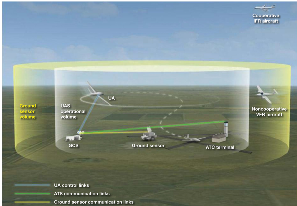
Figure 2. Terminal-area operations access profile. 2 ATS, air traffic services; GCS, ground control station; IFR, instrument flight rules; VFR, visual flight rules.
