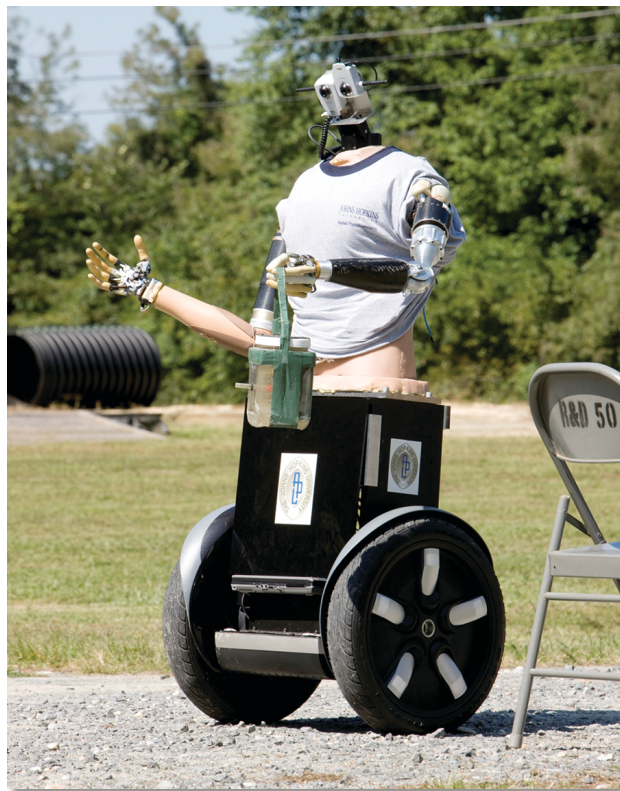
Figure 1. Early human capabilities projection robotic system, Segway Sally, performing an EOD exercise at the Naval Explosive Ordnance Disposal Technology Division (NAVEODTECHDIV) in Indian Head, Maryland.
