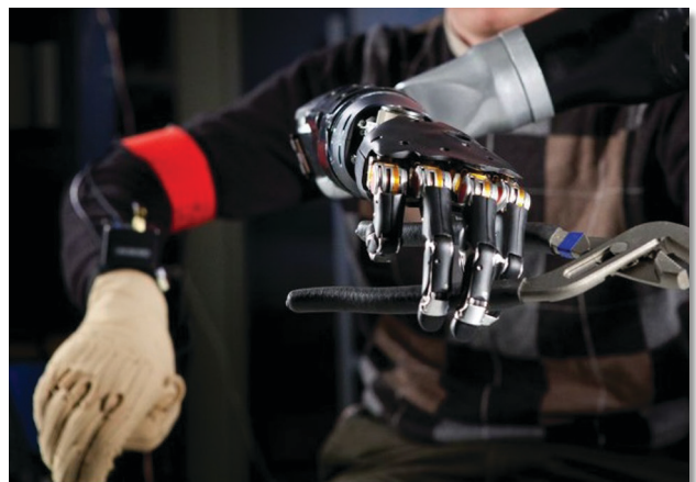
Figure 3. One-to-one mapping of the operator's hand movements using CyberGlove control inputs.
