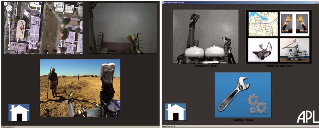
Figure 4. Menus for eye-tracking-based interaction with robotic system. (Left) Contextual mode. (Right) System main menu.
