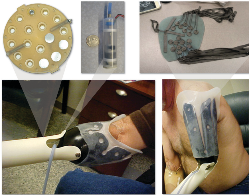
Figure 8. Hybrid base socket with microframe and silicone inner socket. Socket tools that could be used to enhance the base socket are shown above.
