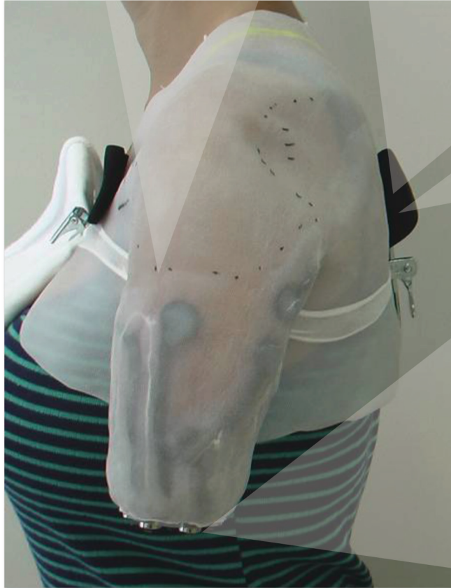
Figure 7. Upper-arm all-silicone base socket with embedded flexible fabric electrodes and a socket common connector plate. Areas of other socket tool use are also highlighted.
