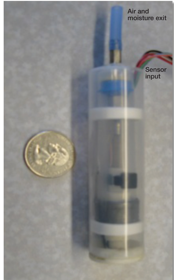
Figure 14. Vacuum control tool for generating negative pressure environments that enhance silicone base socket design suspension. The vacuum control tool was designed in a lightweight, compact, energy-efficient package to pull residual air from between the socket surface and skin surface, creating a suction or negative-pressure environment. This environment increases suspension, reduces shear, and eliminates moisture. As air leaked into the socket interface, sensors in the system would cycle the pump to maintain set levels of negative pressure, resulting in consistent suspension and control.
