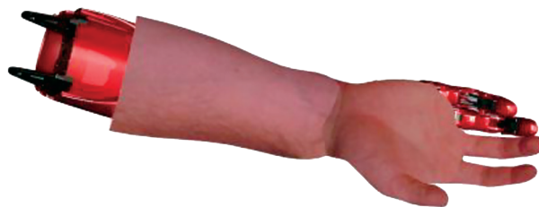
Figure 1. Conceptual lower limb and hand with SG cosmesis (ring and little fingers left uncovered to show detail).
