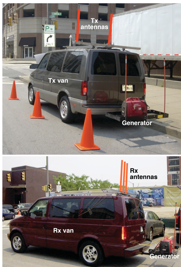
Figure 3. Photos of the transmitter (Tx, upper) and receiver (Rx, lower) vans.
