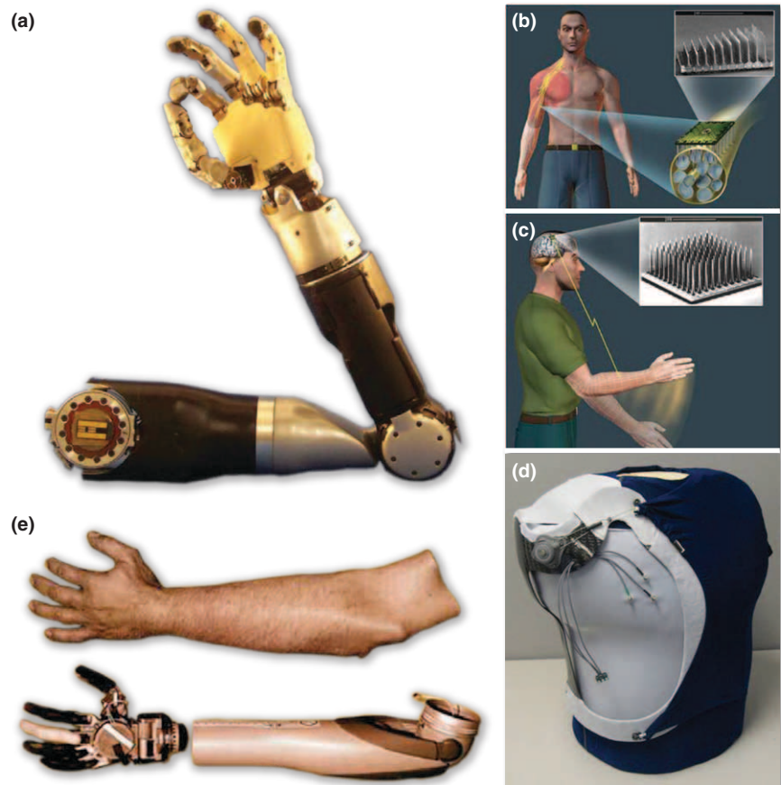
Figure 2. MPL components. (a) MPL upper-extremity prosthesis. (b) MPL peripheral nerve control/feedback using the Utah Slant Electrode Array. (c) MPL cortical control/feedback using the Utah Electrode Array. (d) Body attachment for shoulder disarticulation prosthesis. (e) Cosmesis for upper-extremity prostheses.
