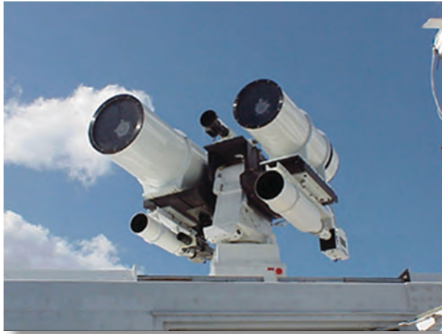
Figure 6. One of the ADOTS camera mounts is shown, deployed above the control van. The mount contains five lenses used to capture still and video images of a missile launch.
