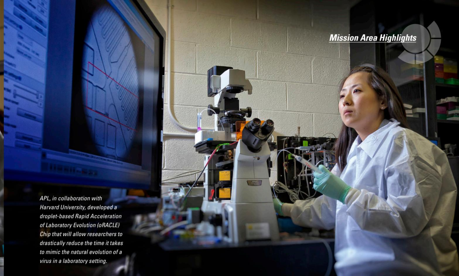
APL, in collaboration with Harvard University, developed a droplet-based Rapid Acceleration of Laboratory Evolution (oRACLE) Chip that will allow researchers to drastically reduce the time it takes to mimic the natural evolution of a virus in a laboratory setting.
