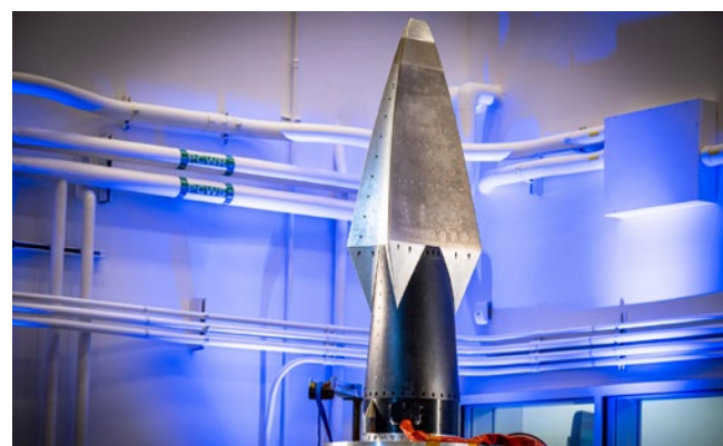
An APL team developed and built the Boundary Layer Transition (BOLT) flight hardware with help from an Air Force research grant. (Credit: Air Force Office of Scientific Research/Johns Hopkins APL)
