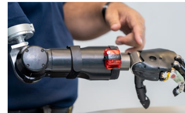
Capable of effectuating almost all of the movements as a human arm and hand and with more than 100 sensors in the hand and upper arm, the APL-developed Modular Prosthetic Limb (MPL) is the world’s most sophisticated upper-extremity prosthesis.
