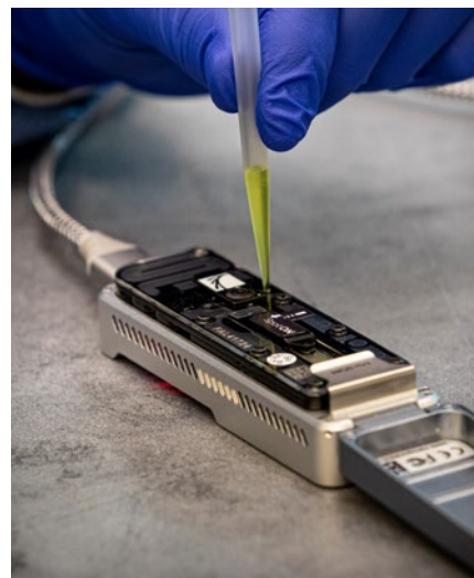
A loading buffer is injected into a handheld DNA sequencer to prepare it for operation.
