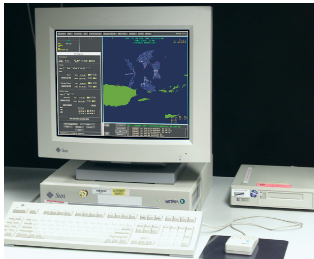
Figure 1. A typical stand-alone CEC display system. Shown here is a Sun Ultra 1 workstation running in a CEC development laboratory at APL. Shipboard systems are similar, with a trackball replacing the mouse.
