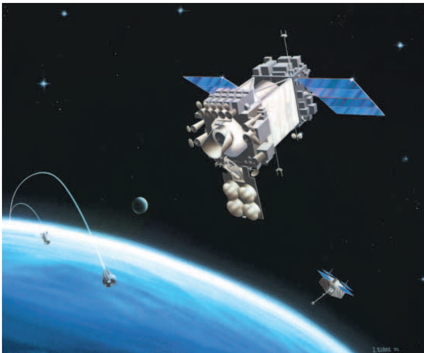
Figure 1. This artist's concept of the MSX spacecraft in orbit includes representations of the principal MSX missions of demonstrating ballistic missile tracking (lower left), cataloging resident space objects (lower right), and collecting phenomenology data on terrestrial, celestial, and Earth-limb backgrounds. The central importance of complete, careful, instrument calibration is represented by the NIST-calibrated reference sphere (left center)—one of six that will be released from the spacecraft.
