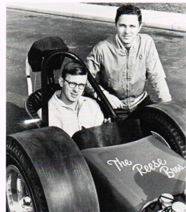
Sitting in the driver compartment of the Chrysler dragster is “Bub” Reese, with his brother Phil standing by. Note that the driver is wearing neither aluminized protective clothing nor a body harness in this posed photo. Clearly seen is the necessarily excessive width of the rear tires, location of the driver compartment aft of the rear axle, the protective roll bar, and the drag parachute. (Photo by John A. Durand.)
