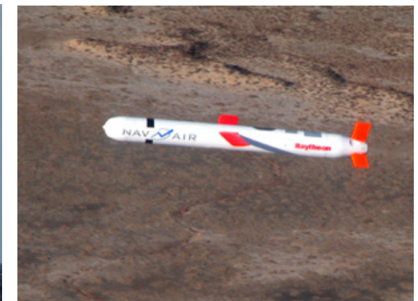
APL's game-changing terrain contour mapping and digital scene matching technologies have ensured greater accuracy for the Tomahawk weapons system. (U.S. Navy)
