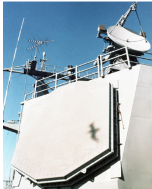
The AN/SPY-1 phased-array radar undergoes operational testing aboard USS Norton Sound , 1980. (U.S. Navy)
