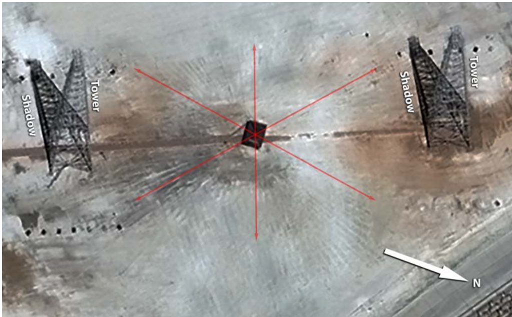
Figure 22. Probable VLF/LF Antenna Counterpoise
